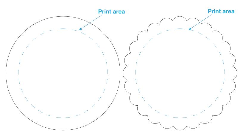
The registration movement is 2 to 3 mm per color in any direction
