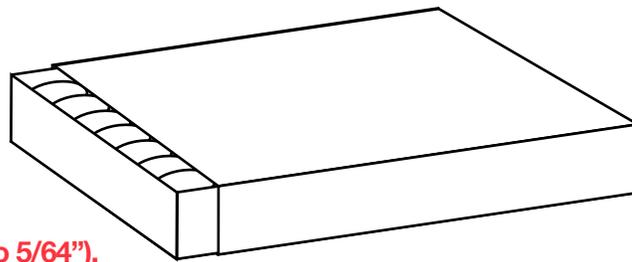
\*\*\*Possible movement of 1 to 2 mm (3/64" to 5/64"), in any direction, during the cutting process.\*\*\*
